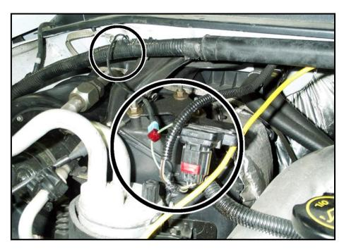
To install the electronic boost cut-off, locate the map sensor located on the passenger side of the engine compartment near the rear. Attach the T-Tap or Posi-Tap to the center wire (Light Green/Black trace) and connect the other end to the chassis ground nearby. This device prevents the SES light (high boost code) from appearing.
